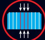
The power of half-cell module increases, and the hot spot temperature reduces because of lower working current
